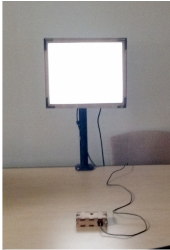
Figure 1: Setup for the rest is construction : un-polarized monitor and custom viewing camera.
